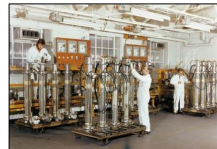
Case Bonded Production of Propellant. Photo Courtesy of BAE.
