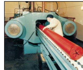
Extrusion Production of Star Web Propellant. Photo Courtesy of BAE.
