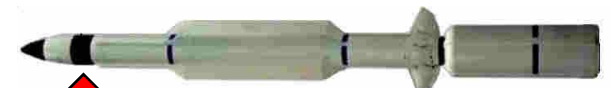
↑ Reaction Jet Divert ( SM-3 3 rd Stage ), SM-3 Also Has Reaction Jet Attitude Control, Tail Control, TVC )
